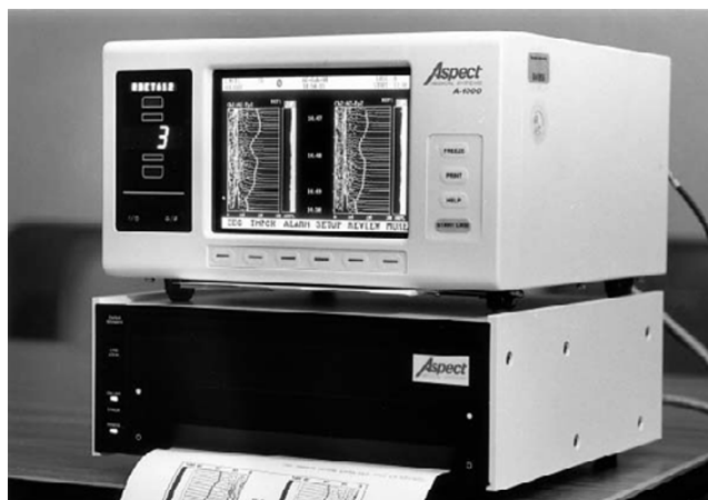
The ASPECT A1000®, a typical brain wave monitor capable of real time bedside EEG.
